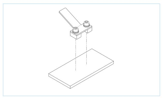
4. Ensure bolt-on is orientated along strain path as shown
