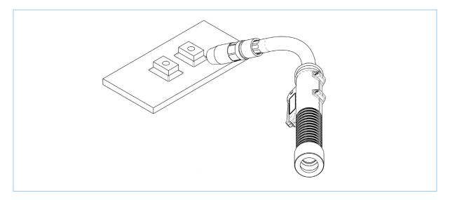
7. Fit the bolt-on sensor to weldable blocks using bolts provided to 10 Nm. Allow 30 min for the bolt-on sensor and substrate to normalise in temperature. Finally, loosen bolts and re-tighten to 40 Nm.
