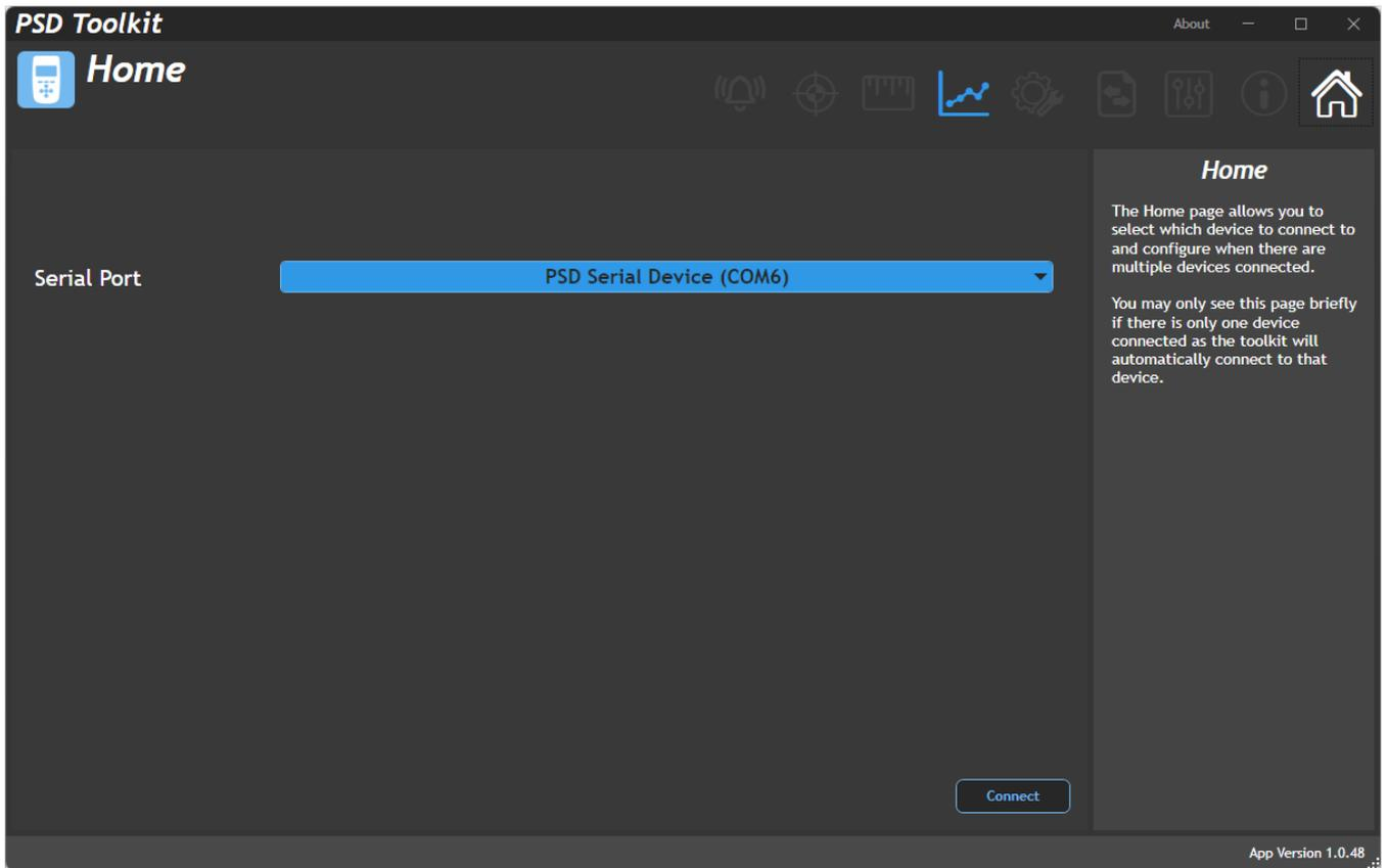
When you connect the handheld to the PC using a USB cable it creates a virtual COM port on the PC. All detected PSD devices are displayed in the drop-down list and you need to select the appropriate one. If only one handheld is detected you may not see this page as the Toolkit will automatically select and connect to it. After selecting the Serial port click the Connect button.
