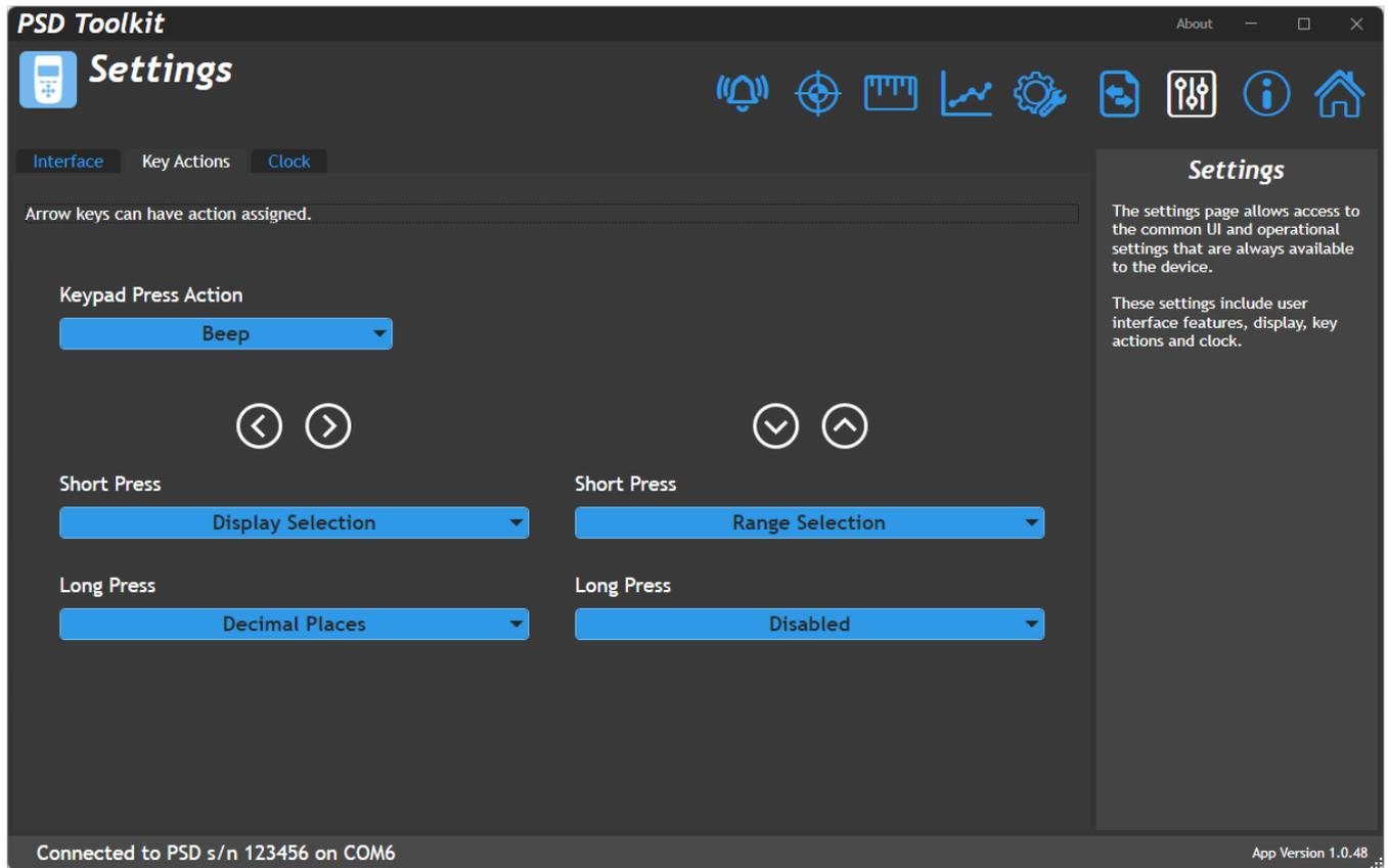
Here you can configure the user interface of the handheld and change settings of the keypad actions and functions.
