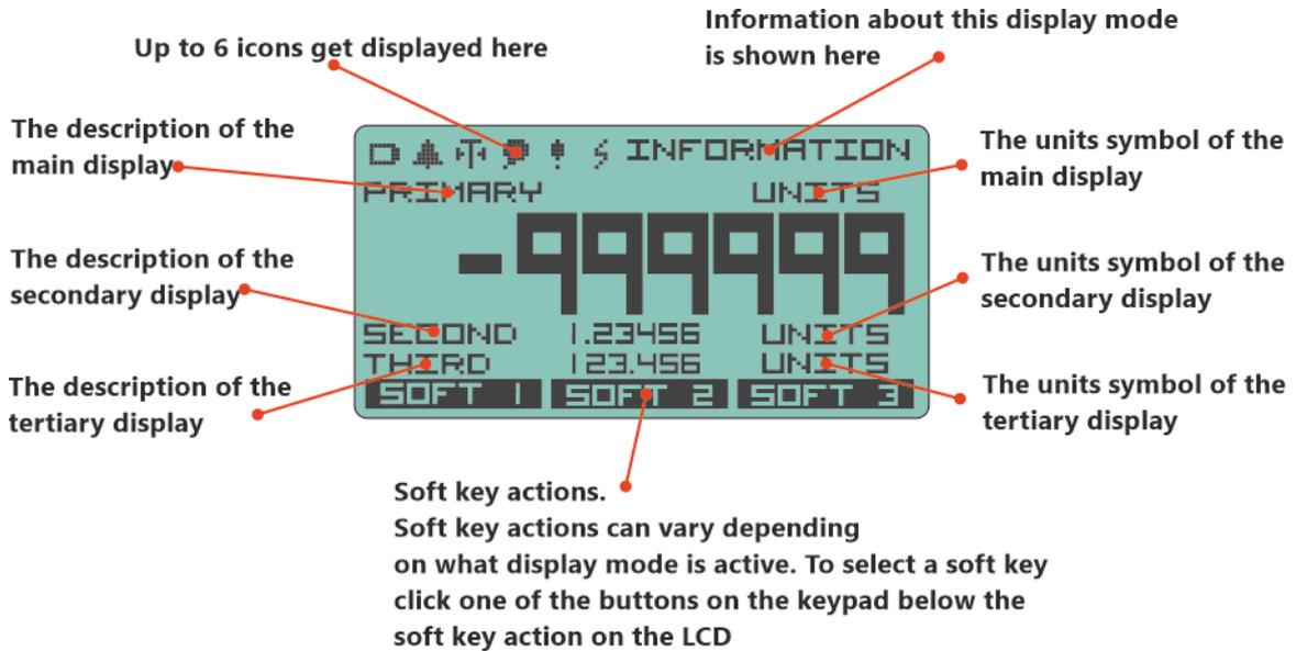
The **values** for the main, secondary and tertiary items are not indicated on the above diagram to improve clarity.
