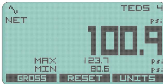
Soft keys allow you to toggle between Zeroed and Gross values and to Reset the min and max to the current value. The usual Units selection is also available.
