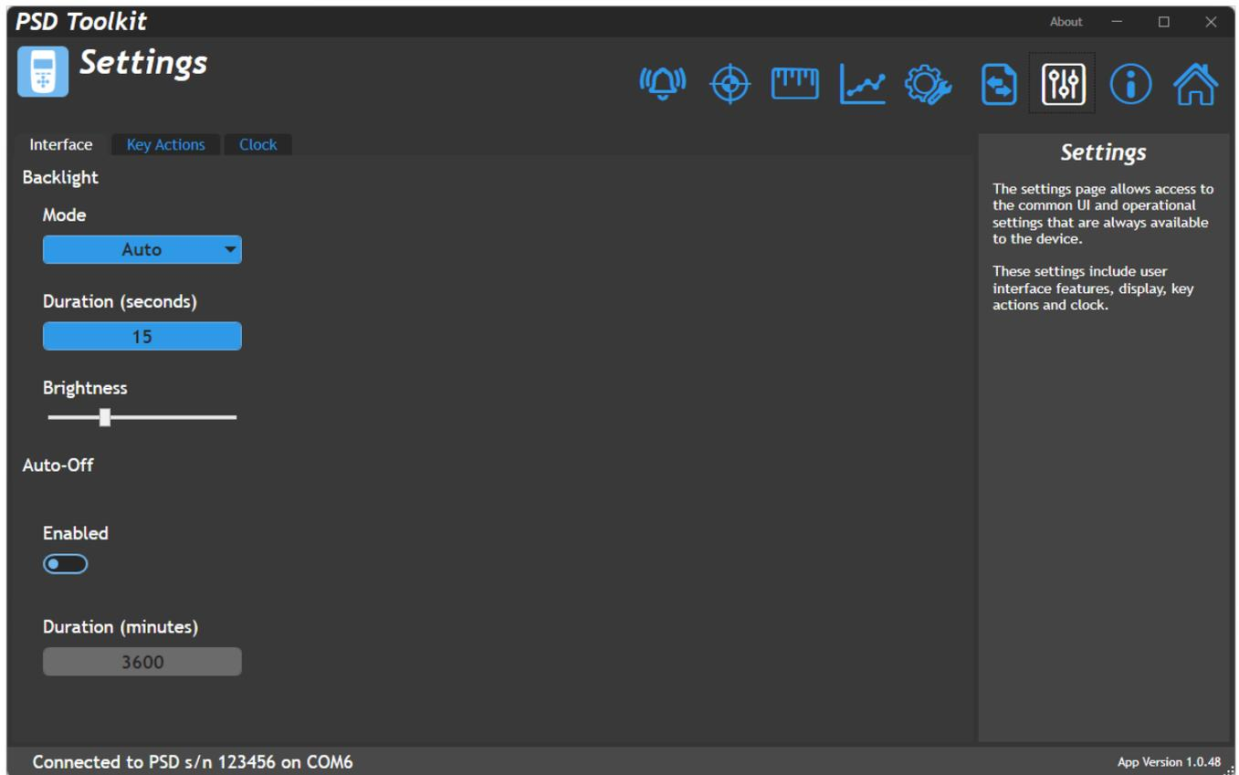
Here you can configure the user interface of the handheld and change settings of the backlight and keypad.
