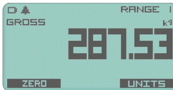
The current calibration range is display top right and Gross or Net is displayed above the main value. Current units are displayed above right of the main value.
