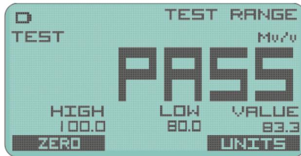
The High limit, Low limit and actual Value are displayed underneath.
