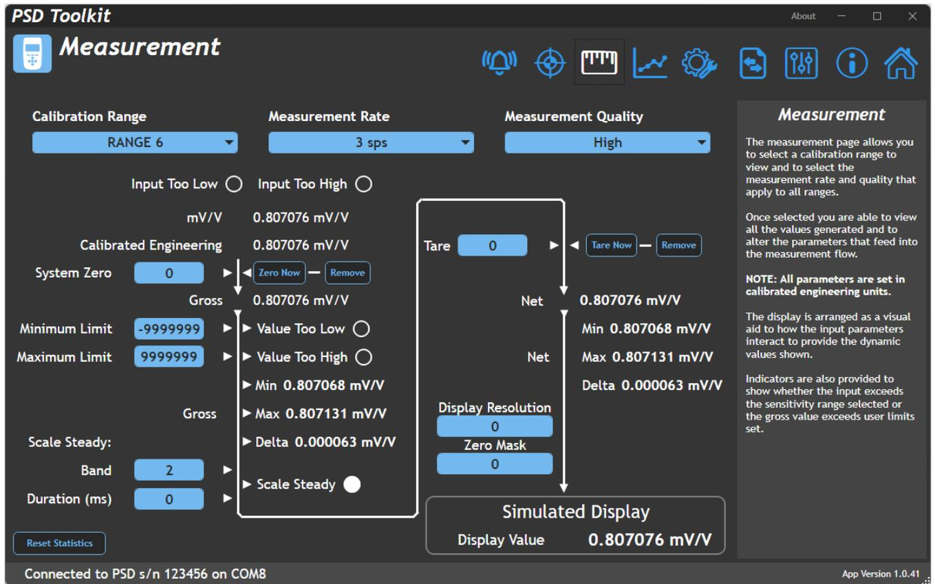
This page allows you to change the measurement settings. It is also presented in a way to visually represent how the parameters interact to generate the various dynamic result values. Each calibration range has its own set of these parameters and they will be remembered the next time the calibration range is selected again.
