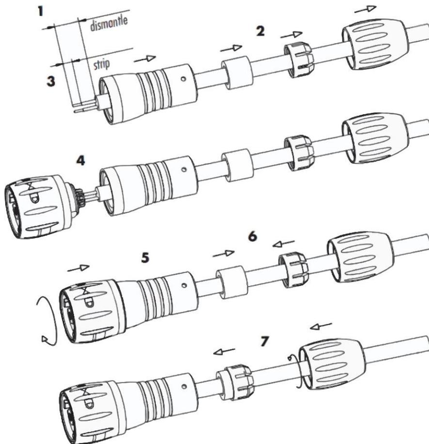
If a cable is already connected to the connector remember to unscrew the cable clamp before unscrewing the main body of the connector otherwise, you risk twisting the cable and breaking the connections.
