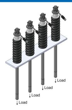
For correct installation, a conical socket and spherical disc must be inserted under the sensor. This makes it possible to compensate for a maximum diagonal pull with a deflection angle of 5° (with a plate thickness of 6 mm).
